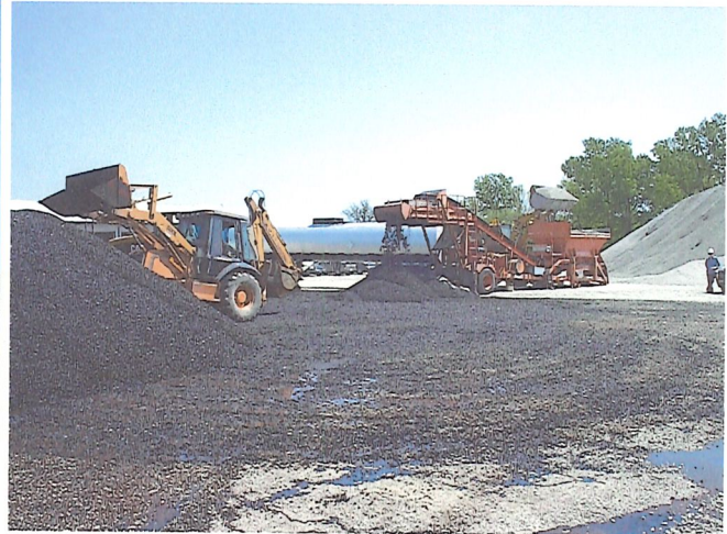
Cold Mix Production at County Highway Department
